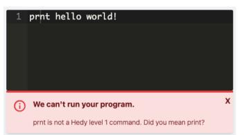
Fig. 6. Misspelling a keyword in level 1 produces an error message that is relatively easy to understand.
